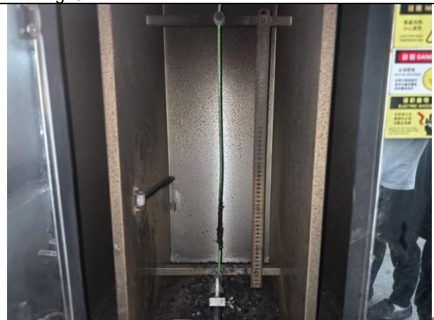
Fig20: Flame Retardant inspection
