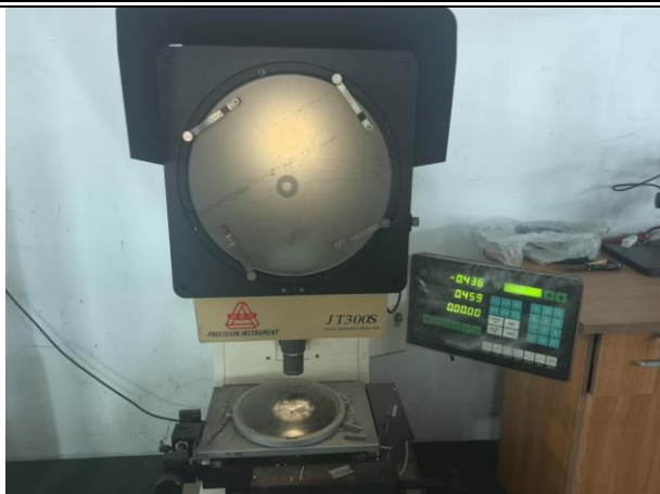
Fig21: Insulation thickness inspection
