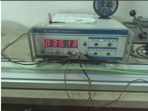
Fig9: conductor resistance inspection
