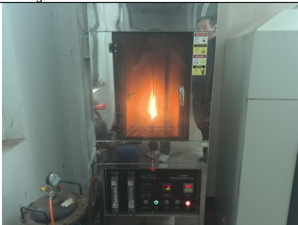
Fig19: Flame Retardant inspection
