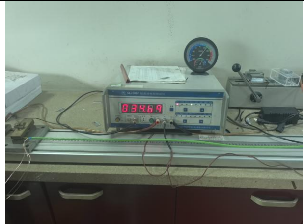
Fig10: conductor resistance inspection
